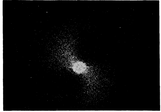
Fig. 19. Fraunhofer image analyzed with the vertical photograph of the surface wave in clear sky by the horogram method.
