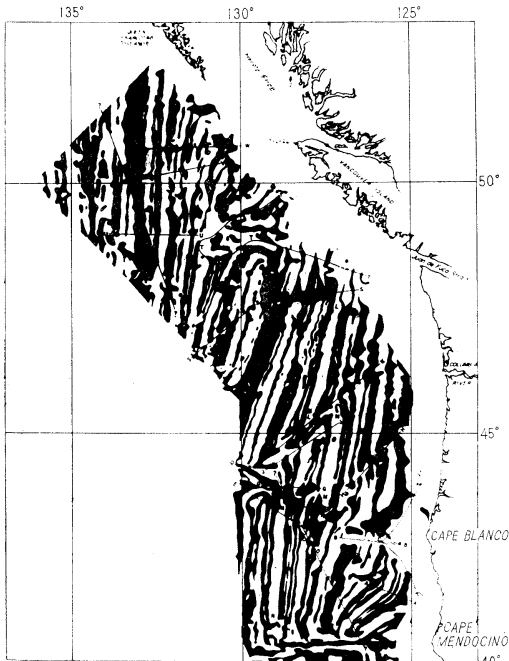
Fig. 9. Index anomaly map of the total magnetic field. The positive area of the anomalies is shown in black. (After RAFF and MASON)
