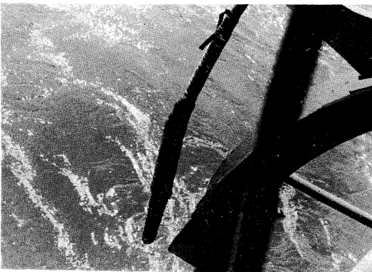
Fig. 6. A sparker electrode used on the Chain.
