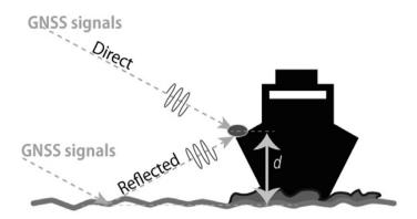
Fig. 2 Concept of GNSS-Reflectometry.
